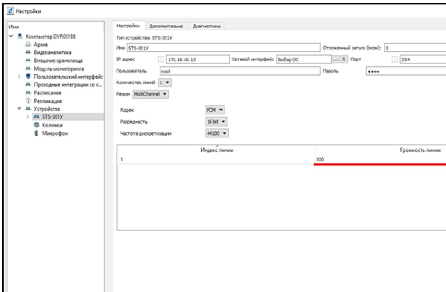
The image shows the "Настройки" (Settings) window for the STS-301Y device. The left sidebar shows a tree view with "STS-301Y" selected. The main area has tabs for "Настройки", "Дополнительно", and "Диагностика". The "Настройки" tab is active, showing various configuration options:
